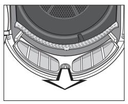
Hold the dial and pull the fluff filter forwards to remove it.
